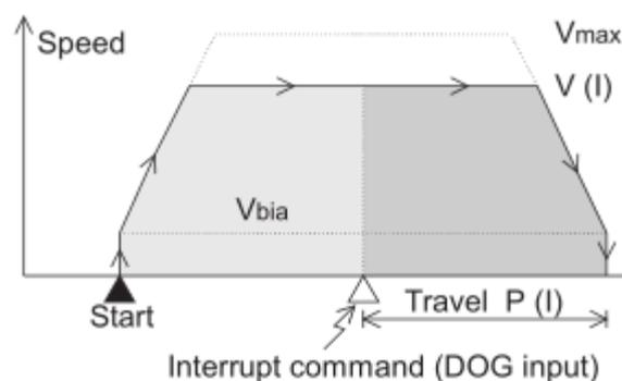
When the start command is received, the motor starts operation. When the INTERRUPT input is received, the motor moves by the specified distance, then stops (The relative travel exclusively can be specified.) The current value is cleared by the start command. The current value starts to change
