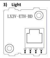
**POW:** power light, normal state is always bright when connected.
