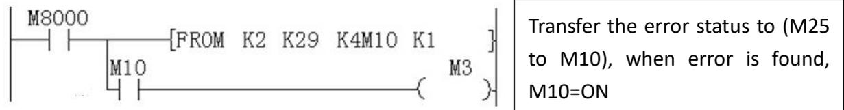
This step provides optional monitoring of the LX3V-4TC Error Buffer Memory (#29). If there is an Error on the LX3V-4TC, bit b0 of BFM #29 will be set on. This can be read by this program step, and output as a bit device in the PLC (Y010 in this example). Additional Error devices can be output in a similar manner, e.g. b10 BFM #29 Digital range error. (see example 3)
